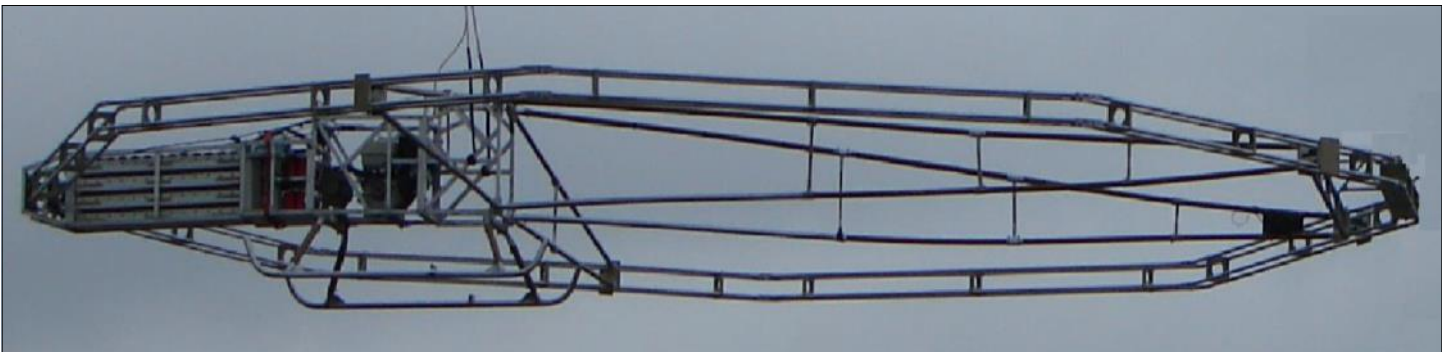
P-THEM comprises an 8.5 metres diameter (57 m 2 ) transmitter loop assembly. Power for the P-THEM system is provided by a motor generator mounted on the transmitter assembly.
